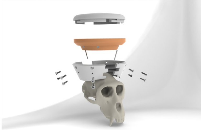
FIGURE 4.29: Headcap system for housing batteries and wireless system.
