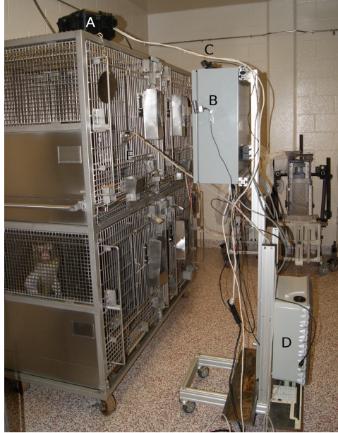
FIGURE 4.31: Home cage wireless recording and behavioral setup. A, Bridge in a waterproof Pelican case;. B, Housing for monitor and computer. C, Webcams. D, Juice bottle case with pump. E, Juicer with IR detector.
