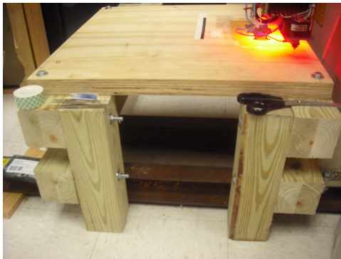
FIGURE B.5: Work table assembled of pressure-treated 4x4 lumber. Table tends to move with varying humidity and temperature, but system is stabilized by video feedback.
